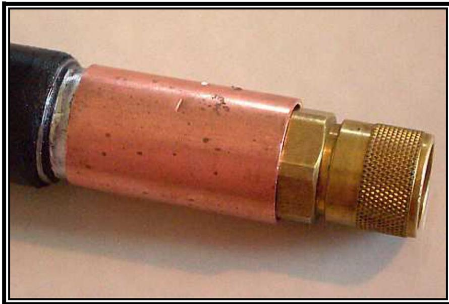
I put a small slit into the side that slips over the aluminum side and tighten it down with a small SS hose clamp. After that I seal it all up with RTV and I'm good to go. If there is anyone interested I can share some images and words of some homebrew 75-ohm to 50-ohm transformers I made for this HL. That's all for now, I hope this will help someone.
