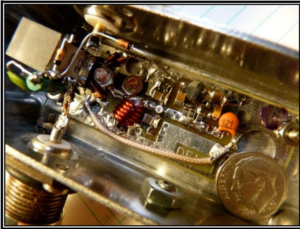
By the way, surface mount turned out to be no real problem. I was able to fit a relay and a bias tee in the same box with a little modification of the board so that it could be mast mounted. From first try it's got enough gain I will probably attenuate it a bit, and we'll see how that helps in the contest next week.
