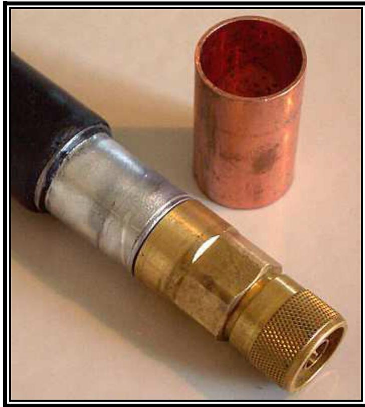
I then slip a 2" long copper coupler (I think it was a 3/4" coupler) over the seam where the two meet and solder them shut at the connector end. You can't solder the copper coupler to the aluminum but it does solder nicely to the brass helix connector.
