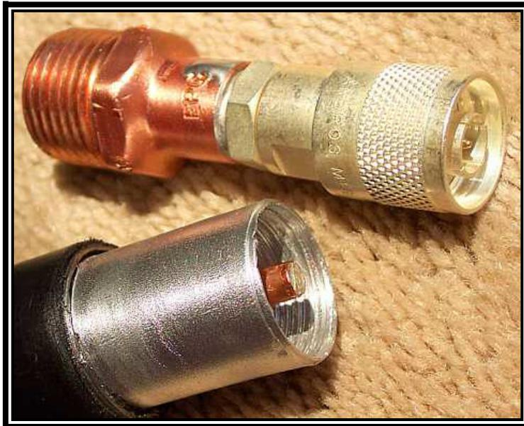
Here is another way. It turns out that the center pin from a regular 1/2" 50- ohm Helix connector fits perfectly over the center conductor of the 75- ohm hard line. It's an absolute perfect fit. The reason is because the difference in impedance's between the two. If this were 1/2" 75-ohm HL this idea would not work. Anyway, solder the center pin onto the center conductor of the HL and assemble the shell of the connector as per normal install. Here is what it looks like:
