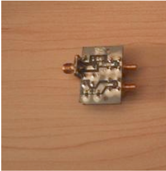
Figure 1: "Connectorized" SRA-11 ripped out of a Ku-band upconverter. The SMB connectors came on the board already installed, plus I got a pad on the LO for free! This is perfect for any L or S-band applications.
