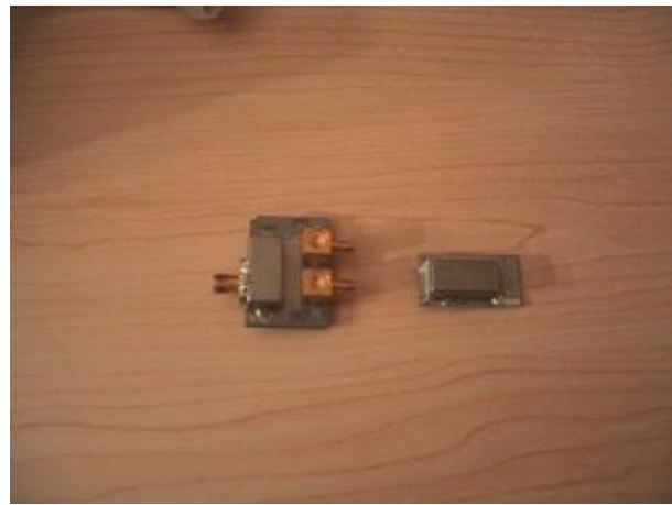
Figure 2: Two mixers ripped out of surplus boards. The one of the left has been retrofitted with connectors, the one on the right has not.
