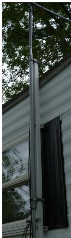
When down, the antenna tops out at about 14' but it can extend up to 26', and it cost about \$.50 per foot for materials. This sort of arrangement works fine for light antennas like Moxons, Cheap Yagis, and the Mini Horse. When bad weather threatens, its easy to lower or remove altogether. I hope these ideas may be useful for a few hams, either roving or at the shack.
