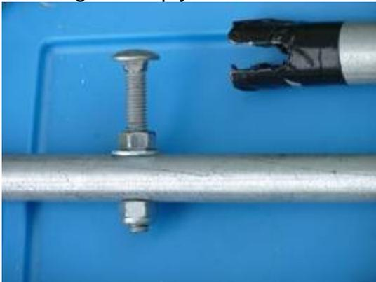
So, I put a 1" deep notch in the top of the main mast where I can reach up and hang a shorter sub-mast on a 5/16" bolt. The sub-mast carries a 28" top tube with 1 or 2 antennas mounted, and a lower 48" tube slides up into place with 3 more antenna mounts.
