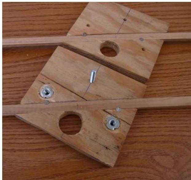
A hole for the mast was drilled through the blocks, and a 4" angle iron, mounted on the pivot bolt, attaches to the mast with a hose clamp.
