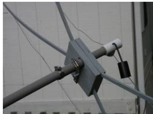
The corners pass through a short piece of vinyl tubing that fits snugly over the strip ends, and the line is knotted at each tube. The whole array can easily flex to mount the corners, and it then has about 5-6 inches of bow, elevating the plane of the wire above the blocks. Gray spray on primer renders a stealthy, non-gloss finish.
