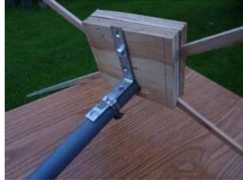
Two 1/4-20 T-nuts set in the upper block allow thumb screws (carriage bolts in photo) to lock the blocks into alignment. Loosening them with the mast out allows the strips to rotate parallel, folding flat and compact.
