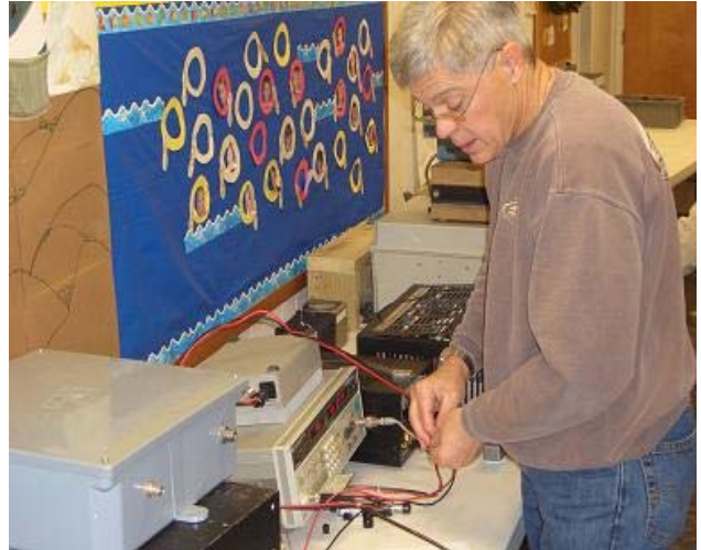
Power measurement and noise figure stations
