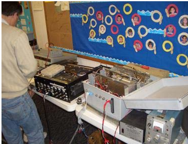
Dave K2DH, John WB2BYP, and Bill K2TER doing power and noise figure measurements.
