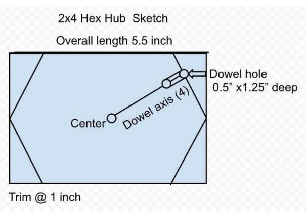
From hub center, draw a line perpendicular to each face cut line, this is the dowel axis. When you make the face cuts, extend the axis line across the cut and mark the center for the dowel hole. Drill a  $\frac{1}{2}$ " hole 1  $\frac{1}{4}$ " deep perpendicular to the face. I would suggest reaming this hole with the drill a little so the dowel fits easily, it will swell when wet.
