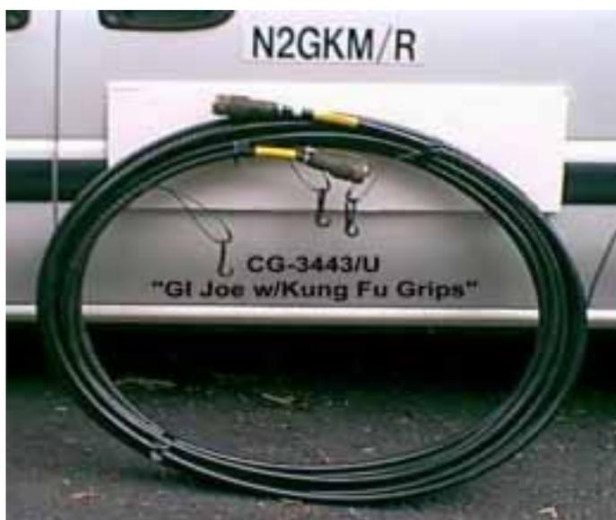
This cable assembly is better known to the Military as CG-3443/U NSN 5995-00-144-0228. The 20 lb. 80’ Coax Cable Assembly (shown above) is terminated with very large male connectors. The photo ON THE COVER OF THE SEPTEMBER VHF JOURNAL shows a close up of two of the connector ends, one with, and one without, the attached protective cap in place. I’m told the connectors are a member of the LQ family.
