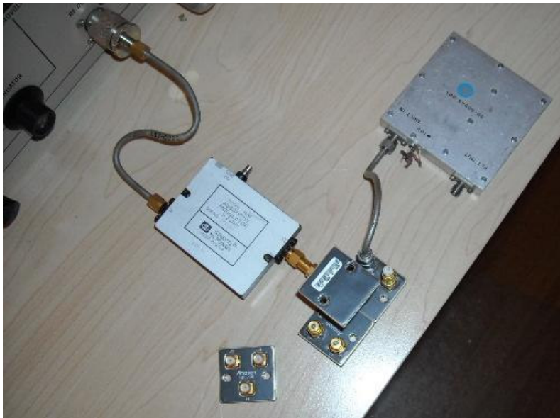
The 3456 multiplier. Keying is provided by supplying -5VDC the unused port of the absorptive modulator to turn off the RF. The Multiplier/Amplifier block takes +10V (though 13.8 seems to work fine). The multiplier is capable of around +12dBm at saturation. While I have a power oscillator providing the input here, a stabilized 1152 MHz oscillator would provide the RF in actual service. This could be a ovenized "brick" oscillator, or perhaps a GPS-disciplined oscillator of some sort.
