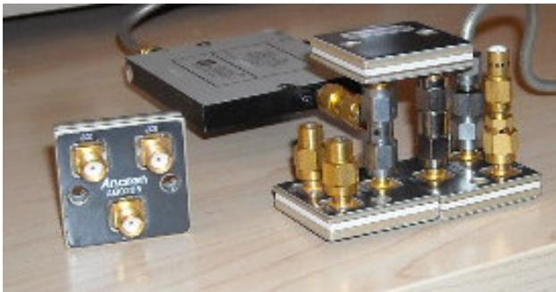
**Closeup picture of the 4-way splitter using three hybrid splitter/combiners. The first splitter is upside down and feeds the inputs of the two bottom splitters. This creates four 50-ohm ports. I have terminated the unused ports in this picture, but in a complete 4-band system they would each have their own multiplier/amplifier chain. A fourth splitter is shown off the the left.**
